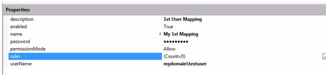
6. Click on the Ellipsis button for **rules** and this will give you an option to add multiple patterns for matching based on certificate properties.
