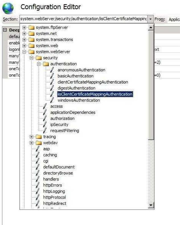
You will see a window to configure Many-to-One or One-to-One certificate mappings here. This is the UI provided through Configuration editor from where we can setup all the mapping configurations.
