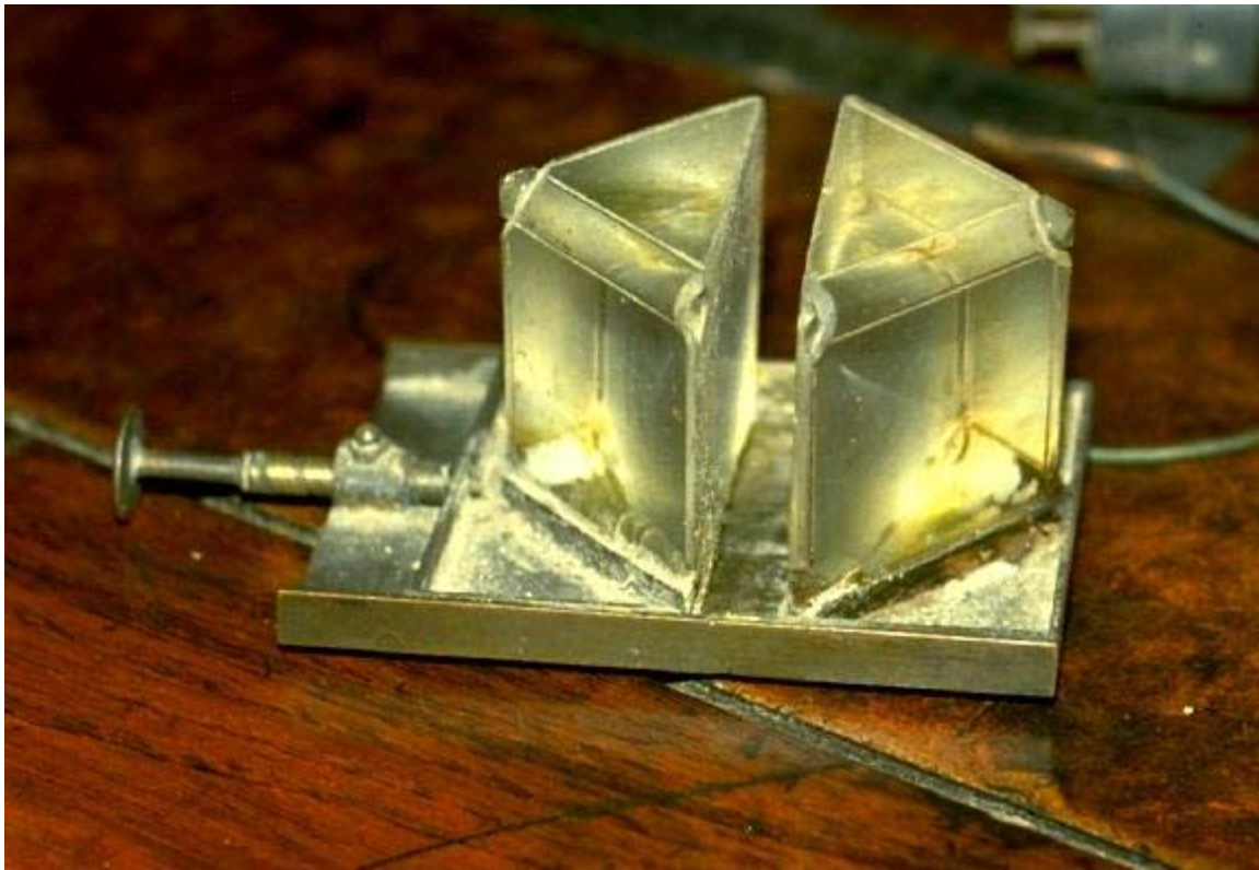
Figure 14. One of Bose's original double-prism attenuators, with adjustable air gap.
